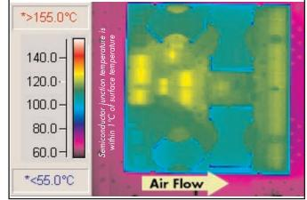
Figure 6: Thermal plot of converter at 30 amp load current with 55°C air flowing at the rate of 200 LFM. Air is flowing across the converter from input to output (nominal input voltage).
