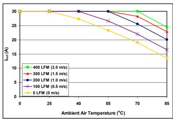
**Figure 5:** Maximum output power derating curves vs. ambient air temperature for airflow rates of 0 LFM through 400 LFM with air flowing from input to output (nominal input voltage).
