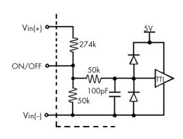
Figure B: Internal ON/OFF pin circuitry
