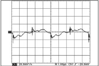
Figure 16: Output voltage ripple at nominal input voltage and rated load current (20 mV/div). Load capacitance: 1µF ceramic capacitor and 15µF tantalum capacitor. Bandwidth: 20 MHz. (See Figure 13)
