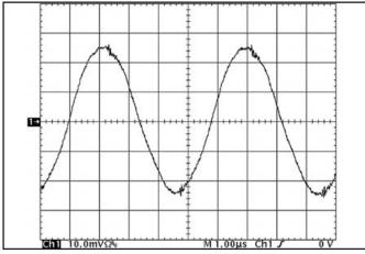
Figure 14: Input Terminal Ripple Current,  $i_c$ , at full rated output current and nominal input voltage with  $10\mu H$  source impedance and  $47\mu F$  electrolytic capacitor (100 mA/div). (See Figure 13)
