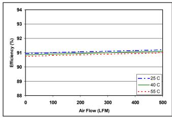
**Figure 2:** Efficiency at nominal output voltage and 60% rated power vs. airflow rate for ambient air temperatures of 25°C, 40°C, and 55°C and nominal input voltage.
